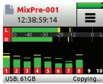
**Do not remove the USB thumbdrive from the recorder when Copying is in progress.**
